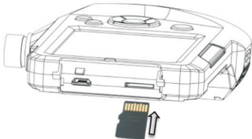
Insert card : Power off the device, open the cover on the backside of the monitor and insert the TF card according to this chart.
